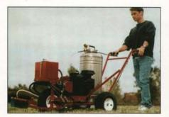
The BS2000 drives forward and reverse with adjustable speed control up to 4 miles per hour. A 12-gallon stainless steel tank reduces the number of delays for refilling. Standard equipment on the BS2000 is a fully adjustable spray box and a 12-foot handhose with wand. The spray box is offset to eliminate straddling of freshly painted lines. Pioneer Manufacturing, Co., Circle number 136 on postage-free card
