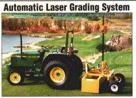
For level, single, or dual grade, **GRADEMASTER** is <u>auto-</u> <u>matically</u> laser controlled and eliminates uneven grade, potholes, wet spots and dips on athletic fields, greens or tee boxes. **GRADEMASTER** . . . The Right Choice for your Grading applications.
