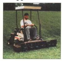
Designed for 700 and 900 Series power units, Grasshopper's 40- and 60-inch AERA-vator™ attachments aerate turf and relieve surface compaction without irrigation, leaving no cores to clean up. Turf is available immediately after treatment. Oscillating, forged-steel tines penetrate and fracture hard, dry soils, encouraging root development and providing a resilient surface for playing fields.
