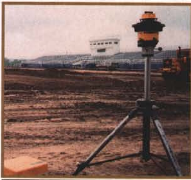
Laser levels offer excellent accuracy and can be operated by a single user.
