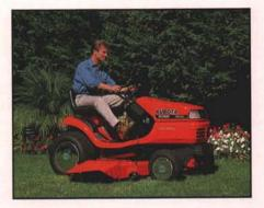
precise control without appreciable loss of horsepower in turns. Other features include Kubota's Cushion Ride suspension system, a clutchless hydrostatic transmission, and choice of 48or 54-in. cutting decks.
