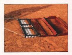
The basic 2-section model, pulled by hand without weights, quickly grooms base lines and infields. Add the scarifier/ballast box section and weights, and attach to any standard lawn and garden tractor, and you can cut 1-in. into the soil to improve rough fields.
