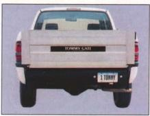
and consists of Grade-A, extruded-aluminum components that interlock for added strength. The rust-free, streamline design is lightweight and easy to close. This option is available on more than 70 models of the traditional cable series.
