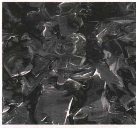
Figure 1. This SEM image shows organic colloids taken from an undiluted liquid humate aliquot. The dark material in the right center of the micrograph is the organic particulate material that has formed on and around the precipitated salt crystals from the bulk solution.
