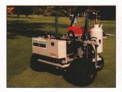
tured by up to 100 psi of air pressure, followed by a short blast of inert, nonbiodegradable, non-toxic polystyrene beads. The beads help relieve compaction and aid in the percolation of water, oxygen, and fertilizer.
