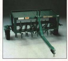
tors to add as much weight as required to penetrate heavily compacted soils. Its 48 hardened-steel tines stretch 42 in. across, and cut holes 3/4 in. in diameter and 4 in. deep.
