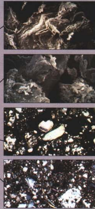
Figure 2. Micrographs imaged in cross-polarized light provide micromorphic detail to a profile diagram of a sports turf rootzone construction. Micrograph A (top) illustrates a layer of fine-grain quartz particles with carbonate cementation and remnants of amorphous iron sulphide framboids indicative of black layer occurrence. Micrographs B-D illustrate a cemented layer at 80-100 mm range. Note differences in grain sorting at the upper boundary illustrated in B and the lower boundary illustrated in D.
