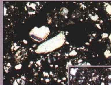
Figure 3. Thin-section micrographs in cross-polarized light show two different synthetic-fiber rootzone
