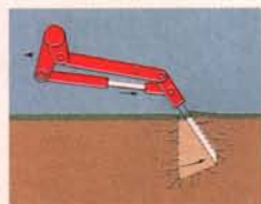
Verti-Drain's patented parallelogram design shatters the soil. Coring tines are also available on all models.
