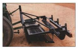
A pioneer in field grooming is proud to present the Diamond Demon Big Boy and Varsity models three point hitch series. These models plow, pulverize, drag, roll and brush finish. The Big Boy will furnish a big 76" wide finish to your ball diamond and will even work on tractors with a 6' tire span. The Varsity model offers a 54" working width and includes the same five functions as the Big Boy, but is designed for tractors with a 48" wheel span. (Kubota, Small Ford, John Deere, etc.)
