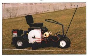
The Jaydee Drive Liner is a self-propelled riding line marker. The 35-gallon paint tank carries enough marking material for a complete game field, or several practice fields. The 2-gallon flush tank cleans the discharge lines for work breaks, travel, or overnight. The center or side-mark spray shields are always operator-visible. A nearly zero turning radius reduces or eliminates back-and-turn maneuvers.
