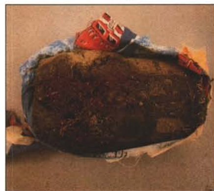
This soil core has been treated with a dipyrldyl indicator solution. The red staining on the core indicates the presence of reduced iron.
