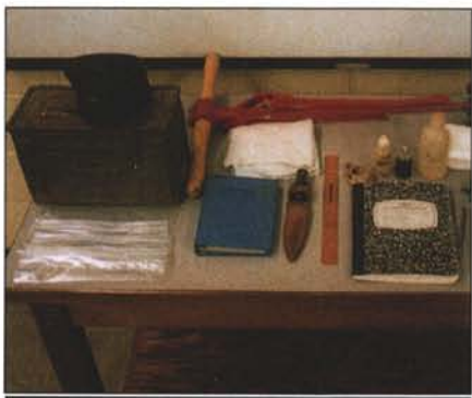
A field soil tool kit includes a cup cutter and a box large enough to hold a camera, color charts, thermometer, spray bottle, chemicals and other items. Photos courtesy: Michael DePew.
