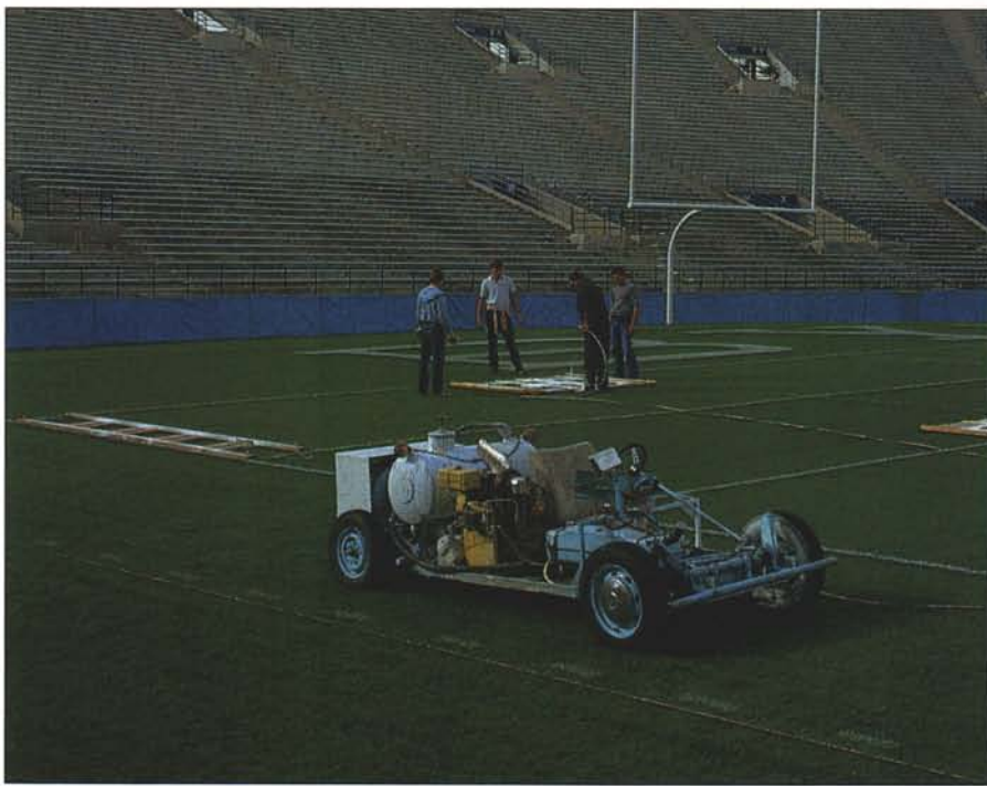
The main delivery system used at BYU is a modified four-wheel VW buggy.
