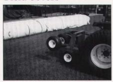
Covermaster, Inc.'s Tarp Machine, now at less than half the price of the original model, rolls out large athletic field covers. To use, hook up the portable unit to any standard tractor equipped with a minimum 14 hp and 540 power take off (PTO) unit.
