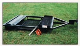
The Diamond Demon ... a revolutionary new machine designed to put your baseball or softball fields into great shape with a minimum of time and effort. The Demon plows, pulverizes, drags, and rolls the field in one simple operation. Diamond Demon will produce a level playing surface, soft enough to be safe, yet firm enough to provide the excellent surface every coach looks for.
