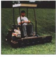
Designed for 700 and 900 Series power units, Grasshopper's 40- and 60-inch AERA-vator™ attachments aerate turf and relieve surface compaction without irrigation, leaving
