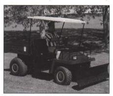
independent coil springs over heavyduty hydraulic shock absorbers. The unit has a wheel tread of 36 inches in the front and 37.5 inches in the rear.
