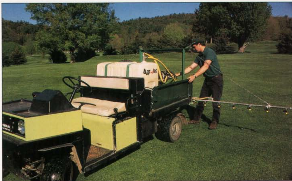
Turf equipment mechanic Andy Bates checks the switches on an electrically operated control he installed to update a turf sprayer. Photo courtesy: Alan Ginsburg.
