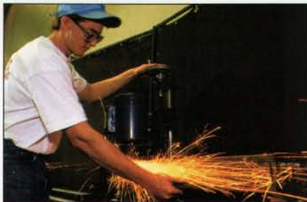
SUNY Cobleskill student Jason Burroughs grinds a bedknife from a reel unit on a Neary grinder. Photo courtesy: Larry Abrams.
