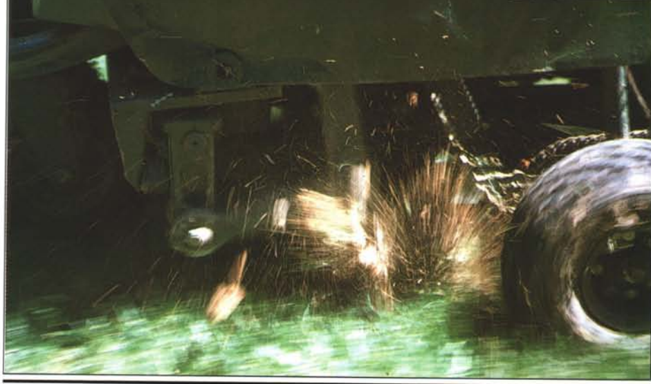
The dirty environment and the severe vibrations of aeration place the machinery involved under a great deal of stress, so regular maintenance is mandatory. Photo courtesy: Trusty & Associates.
