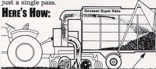
**1** Rotating flails pulverize cores separating thatch from the soil.
