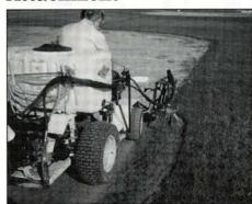
The Kromer Co., of Mound, MN, has developed a new attachment for its popular Athletic Field Maintainer (AFM). Due to incorrect infield maintenance, a dangerous ridge of infield material is often hidden by the grass around the skinned area of ball diamonds. The new attachment, designed to remove this ridge, is a rotary hydraulic-driven nylon bristled broom that spreads this ridge to the infield where it is leveled by the broom attached to the AFM vehicle.
