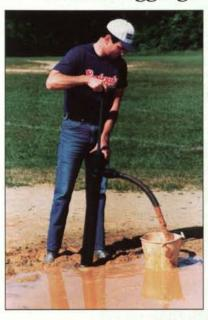
The Diamond Pump is a durable, nonclogging hand pump which easily removes 18-20 gallons of water minute from dirt infields, sand traps, ditches. Made of tough ABS and PVC, a six-inch aluminum disc prevents mud from being drawn directly into the pump. Absolutely will not clog.
