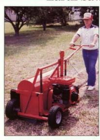
The all new Model K-T 2400 Triple V-Belt Drive Disc Blade Trencher. Ideal for the professional contractor, groundskeeper and golf course superintendent. Financing available. Digs 2", 3" or 4" wide; Adjustable to 12" deep; 20 to 30 feet per minute; Powered by 8.0 hp; Honda-OHV Engine. Root Pruner • Trencher · Asphalt Cutter Guaranteed to outperform in digging
