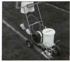
The Trumark Athletic Field Marker is designed for safety, convenience and economy. Mark fields all day with the 12volt deep-cycle marine battery. Dual nozzle spray head provides a distinctive line from two to six inches wide in a single pass. The fold-down handle is convenient for storage and transportation. Ten-inch pneumatic tires on ball-bearing hubs provide rolling ease. The Trumark field marker is safe to use because there are no combustible fuels, pressurized vessels or canisters.
