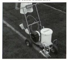
The Trumark Athletic Field Marker is designed for safety, convenience and economy. Mark fields all day with the 12volt deep-cycle marine battery. Dual nozzle spray head provides a distinctive line from two to six inches wide in a single pass. The fold-down handle is convenient for storage and transportation. Ten-inch pneumatic tires on ball-bearing hubs provide rolling ease. The Trumark field marker is safe to use because there are no combustible fuels, pressurized vessels or canisters.
