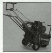
The models TA-19 and TA-26 are roll-type core aerators with 3/4-inch tines that give up to nine holes per square foot and are powered by a four-hp Honda engine.
