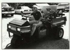
This topdresser will fit in the box of most utility vehicles. A single operator can mount it in the box in minutes, without dismantling any part of the utility vehicle. The unit is self-contained and powered by a five-hp Briggs & Stratton engine. It can distribute top-dressing material from either side or in a full-spread pattern.
