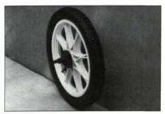
The turf-friendly wide profile is less prone to leaving ruts and will carry heavy loads over soft terrain. The turf tread pattern is puncture-resistant and will give equipment the industrialstrength look. Two sizes of the pneumatic HF224 are available: the 16-by-2.125 size is 16.2 inches tall, 2.1 inches wide and will carry a load of 174 pounds per tire. The 20-by-2.125 size is 20 inches tall, 2.2 inches wide and will carry a load of 213 pounds per tire.
