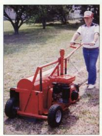
The all new Model K-T 2400 Triple V-Belt Drive Disc Blade Trencher. Ideal for the professional contractor, groundskeeper and golf course superintendent. Financing available. Digs 2", 3" or 4" wide; Adjustable to 12" deep; 20 to 30 feet per minute; Powered by 8.0 hp; Honda-OHV Engine. Root Pruner • Trencher Asphalt Cutter Guaranteed to out-
