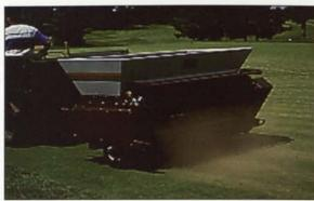
Turfco manufacturing is known best for its production of the Mete-R-Matic line of topdressers. The line includes the large area topdresser for fairways and athletic fields, the non-hydraulic tow-behind topdresser and the selfpropelled walking topdresser. All three units utilize the revolutionary chevron design belt to handle both wet material and light applications. Other products that Turfco produces include sodcutters, an edger, aerators, a soil processor and a sod harvester.
