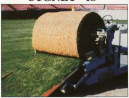
CYGNET is able to harvest 48" wide rolls consistently from very thin to over 2" thick. We can install these rolls without pulling or pushing them along the ground (no stretching or tearing). Our patented machines carry the rolls, turn them at ground speed, and install down a controllable slide for tighter seams. NO ONE ELSE CAN MAKE THIS CLAIM. U.S. Pat. #5,215.248 & 5,307.880.
