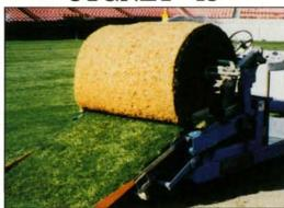
CYGNET is able to harvest 48" wide rolls consistently from very thin to over 2" thick. We can install these rolls without pulling or pushing them along the ground (no stretching or tearing). Our patented machines carry the rolls, turn them at ground speed, and install down a controllable slide for tighter seams. NO ONE ELSE CAN MAKE THIS CLAIM. U.S. Pat. #5,215.248 & 5,307.880.
