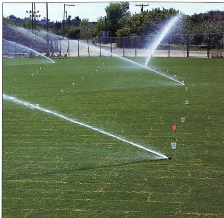
Precipitation rate is measured through catch cans placed near the sprinkler and halfway to the next one. The testing run time should be enough to collect 25 ml of water.
