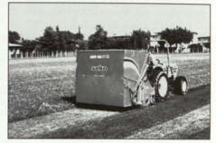
The Seko Super Groomer will dethatch, mow, vacuum, sweep and roll — all in one pass. It will pick up debris such as paper, cans, bottles and small branches. It works well on bentgrass and for athletic-field striping. Units are three-point-hitch mounted with self-contained hydraulics. Available cutting widths are 48 and 60 inches.
