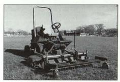
The 60-inch-wide Tine Rake™ dethatcher is designed to fit commercial riding mowers with 60- to 72-inch cutting widths. The dethatcher allows the turf-care professional to remove large amounts of thatch in one operation while mulching or bagging. It does not damage healthy turfgrass. It lifts the grass as it dethatches, resulting in a greener, thicker lawn.
