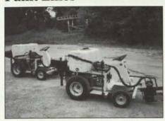
Kromer Company's hydraulic cutter and painter lowers the painted line to below the normal grass surface, so mowing will not remove the painted lines. The lines also last longer on the shorter grass. There is less grass to cover, so the paint coat is heavier. For practice use, the paint may be eliminated or saved as the cut line in the grass is very clear and distinct.
