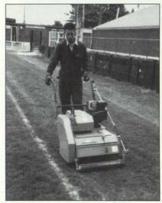
This auto-seeder is a self-propelled machine for rapid overseeding of small areas, such as soccer goal mouths and centers, golf tees, etc. The blades, rotating against the direction of travel, cut shallow grooves 2 inches apart. Seed is placed into the grooves simultaneously.
