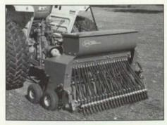
Gandy Company introduces a shoereplacement assembly for its overseeder. Independent spring-loaded shoes follow in the slit created by the cutter blades, and adjust for minor changes in ground contour. Seed placement directly behind each shoe permits more seedmore than 95 percent—to be placed directly into the slit for more seed-to-soil contact.
