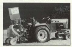
As part of its unique in-soil water management system, HydroGrowth Technology Inc. has developed a series of four installation machines. All are intended for use in a variety of applications, including athletic complexes.
