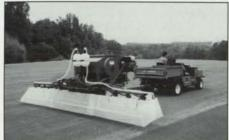
The Course Air Turbo II features a number of improvements, including a 20cubic-foot hopper, breakaway booms for safety, 16- or 20-foot boom spread, shorter tongue for easier turning and lightweight environmental shields. It also has a wide range of application rates — five to 500 pounds per acre for fertilizer, seed or dry pesticides.
