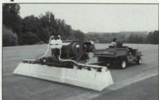
The Course Air Turbo II features a number of improvements, including a 20-cubic-foot hopper, breakaway booms for safety, 16- or 20-foot boom spread, shorter tongue for easier turning and lightweight environmental shields. It also has a wide range of application rates — five to 500 pounds per acre for fertilizer, seed or dry pesticides.
