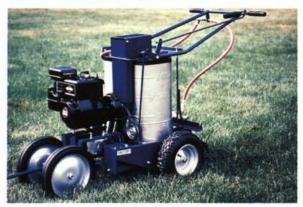
The Jaydee Model 5000 is a fully featured, self-propelled, professional line marking machine. The engine powers a piston pump, providing mechanical agitation, and powers both rear wheels - it tracks a straight line under its own power. The constant 2-mph speed results in uniform line width & brightness as well as predictable marking material consumption.
