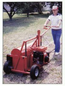
The #1 leader in small disc blade trenchers. Ideal for sprinkler systems, landscape edging, surface root pruning, nightscaping, drainage, electrical lines in conduit, invisible fence. Three Models to choose from (all v-belt blade driven). Forward digging. K-T 200 2" wide Adjustable to 8" deep. K-T 1200 2" or 3" wide - Adjustable to 10" deep. K-T 2400 2", 3", or 4" wide -Adjustable to 12" deep. Kwik Trench stands for quality -performace, service
