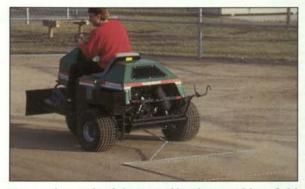
Two-or three-wheel drive sand bunker or athletic field groomer available with: • drag mat • scarifier • leveling blade • rear rake • front blade • 12.5-hp Kubota diesel engine or 16-hp Vanguard V-Twin gas engine • hydrostatic drive • tight turning radius • 10.5-mph transport speed • tilt-up rear engine shroud.
