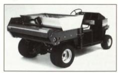
Ransomes America Corporation introduces the Cushman TD 1500 top dresser. When Mounted on the Cushman Turf-Truckster work vehicle, the TD 1500 can deliver high performance and time-efficient top dressing for greens, fairways or athletic fields. The large hopper cuts down the number of time-consuming refills, while the unique conveyor belt design ensures even coverage of top-dressing material. The unit can be operated from the driver's seat by using an auxiliary hydraulic control.
