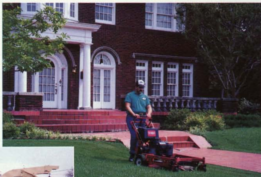
Mulching mowers (above) eliminate the need for bagging and disposing of grass clippings. Photo courtesy: BLT Landscape
