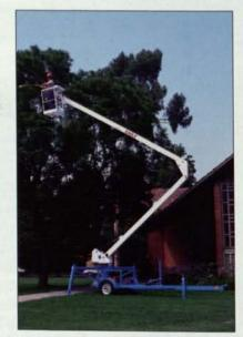
The EAGLE 44, manufactured by AmeriQuip, is a trailer mounted, articulated aerial lift with a 25 ft. side reach and 44 ft. working height. It features positive bucket leveling and 360° continuous rotation.
