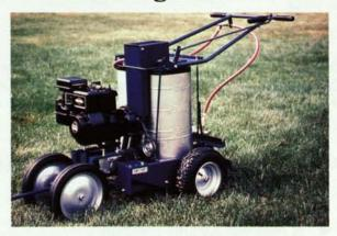
The Jaydee Model 5000 is a fully featured, self-propelled, professional line marking machine. The engine powers a piston pump, providing mechanical agitation, and powers both rear wheels - it tracks a straight line under its own power. The constant 2-mph speed results in uniform line width & brightness as well as predictable marking material consumption.
