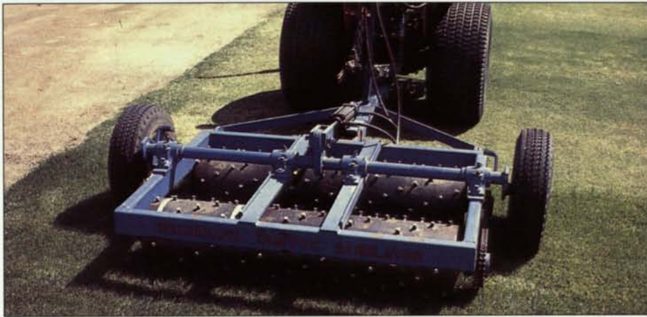
Brinkman Machine used to evaluate wear tolerance of turfgrasses at University California Riverside. Photo courtesy: Stephen Cockerham.
