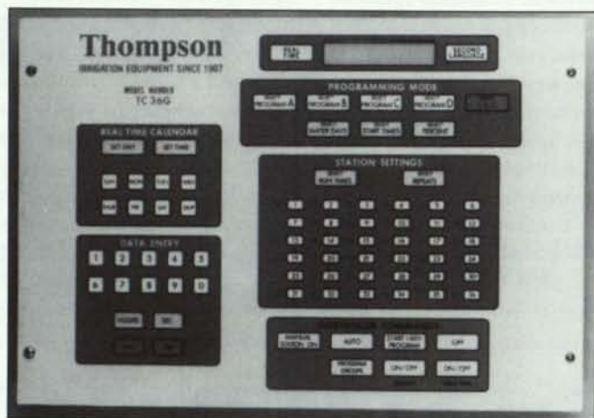
Solid-state controllers have no moving parts and cannot "wear out". Photo courtesy: Thompson Irrigation Equipment.
