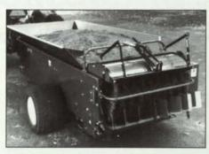
model choice, the blade and scarifier can be raised or lowered individually by manual or electric lift. Brushes give playing surfaces or tracks a perfect finish. Designed as a pull-behind unit with a hydraulic or electric lift, it is ideal for use with most utility vehicles.
