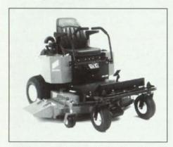
The new Encore PRO-Line rider is user-friendly. This compact hydrostatic rider with zero turning radius is so easy to operate it eliminates the need for small trim mowers. The floating deck allows rough terrain mowing without scalping. The 52" cutting deck features three blades for faster ground speeds.
