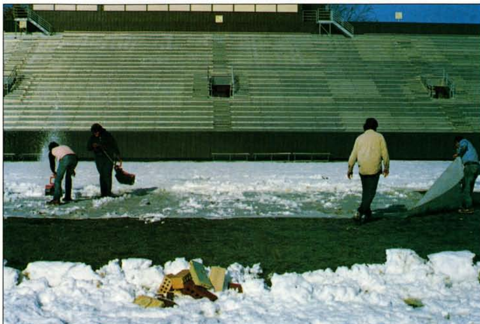
The Holy Cross crew is able to provide a deep-green natural turf field despite severe winters in Worcester with a combination of tarps, fungicides, fertilizers, and charcoal chips.
