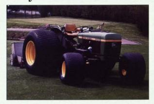
Goodyear 54-3100-26 high flotation turf tire works well anywhere on the golf course, wet grounds or dry. Its large, flat contact area skims over the greens with minimum compaction without rutting or damaging the grass. McCord's custom-built wheels make it easy to convert this tire to your turf equipment.
