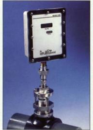
Data Industrial Corporation offers this stand alone unit with 3 to 5 year battery life. This unit is built to NEMA-6P submersion specs. It will continue to operate in a valve pit under 6 ft. of water. It is field or factory calibrated with Data Industrial insertion impeller flow sensors. Handles pipe sizes from 2" to 20" in diameters.
