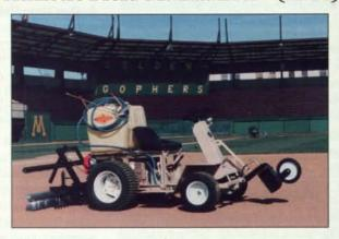
AFM stripes, sprays, and grooms, saving on maintenance time and materials. AFM can stripe several football fields without the need to refill; level and groom athletic fields with a heavy-duty harrow and broom or dragmat; and spray chemicals for weed and insect control. It can also pull a utility trailer or other accessories.
