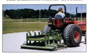
This new diamond groomer is really just a deluxe model of the TRUPLAY. It has all the same tools working for you - the Ripper Blade, Spring-Tooth Rake, Levelling Mechanism, Roller and the Brush. When you're finished no one will know whether it's done by a TRUPLAY or a Diamond-Master. Why do people insist on buying the Diamond-Master? It's better looking. It costs a little more. It's easier to set up and adjust. Maybe they just want the very best. Why not talk to us about it?
