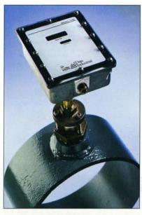
Data Industrial 1400 series flowmeter is a battery-powered insert-style flowmeter that displays rate and total. Display is housed in a rugged aluminum enclosure built to Nema 6P submersion specifications, allowing the unit to operate fully submerged in a flooded meter pit for extended periods of time. The 1400 can be cal-
