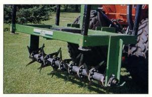
A new multi-purpose aerifier manufactured by Aerway features replaceable bolt-on tines. The well-known Shattertine and the new Finetine are also interchangeable. In the spring or fall, when you want maximum cultivation to over-come compaction, you bolt-on the Shattertines. During the playing season you switch to the Finetines so you can continue aeration in fine turf areas without restricting play. Yes, even on golf courses.
