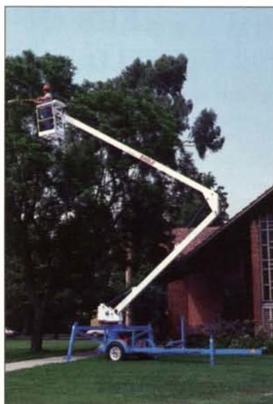
The EAGLE 44, manufactured by AmeriQuip, is a trailer mounted, articulated aerial lift with a 25 ft. side reach and 44 ft. working height. It features positive bucket leveling and 360° continuous rotation.
