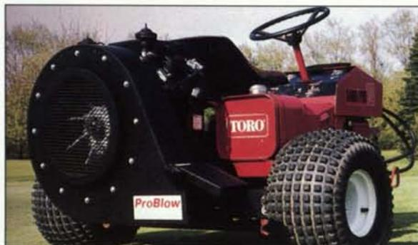
Selbro Inc. offers a high velocity, high output debris blower designed to attach to all popular sand trap rakes. The ProBlow attaches easily to and operates from the fuel and battery of the sand trap rake. The blower is powered by an 18hp twin cylinder Kohler Command engine, and develops over 5000 cfm @ 175 mph. The combination of these two machines creates the most versatile debris blower available in the turf care industry.
