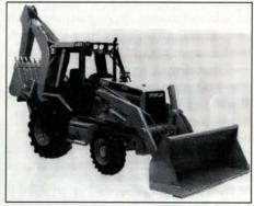
The Caterpillar 446 backhoe loader is updated to a B Series machine. It has a new swing valve for better modulation and control. Increased cylinder capacity provides more hydraulic power and faster performance. Swing torque is increased by 16 percent, improving back-filling and sweeping and swing on a grade.
