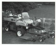
The Multipurpose Exmark Explorer II has a 52-inch floating cutting deck. The deck's TriVantage design enables the operator to mulch, bag, or discharge. The Micro-Mulch accessory recycles clippings into the turf. The rear utility box is ideal for transporting tools, plants, and other materials.
