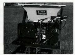
Terracare's skid-mount topdresser will fit on most utility vehicles. It is fully hydraulic, with a variable speed on the feed auger and the spinners. It is powered by an 8-hp Briggs & Stratton engine. **TERRACARE PRODUCTS COMPANY INC.**
