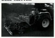
The 4-foot Multislit has five slitting blades fitted to each of eight large diameter plates. The tine plates have a wide rim to reduce marking when working at full penetration. Six- or 8-inch sharpened slitting blades are available for use on fine turf areas such as golf greens, and 6-inch heavy-duty slitting tines are available for outfield turf.
