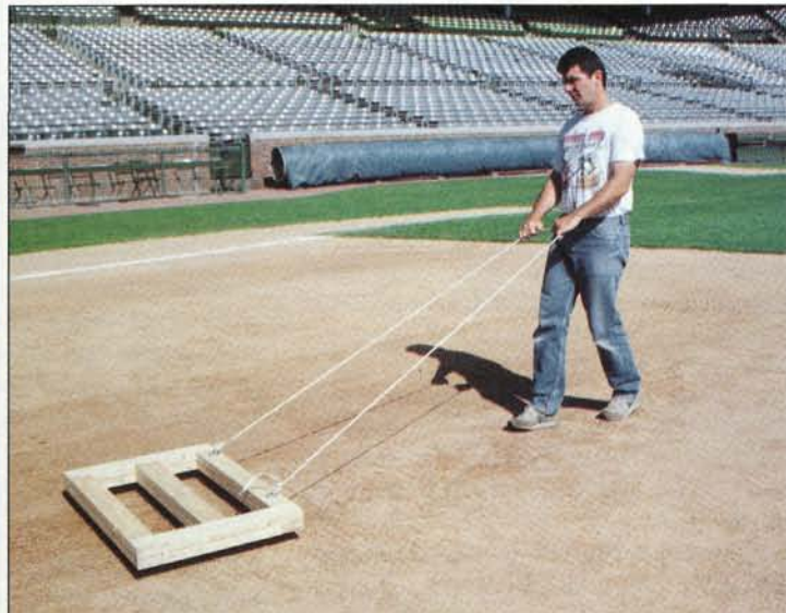
A nail drag should be used a minimum of once a week, more frequently if possible. Photos courtesy: Aimcor.
