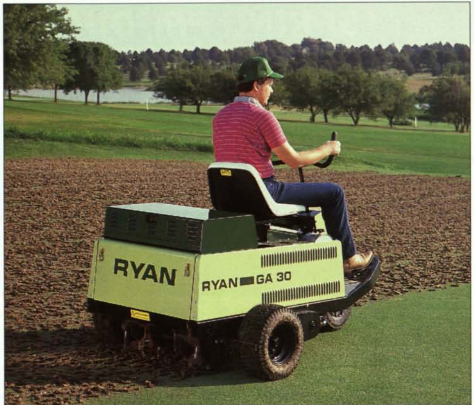
Riding aerator with hollow tines at work. Photo courtesy Ransomes America Corporation.
