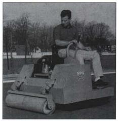
The Auto-Trugreen mower for fine turf allows a higher cut, which increases pace with less stress on the turf.
