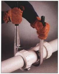
Stamos Tool, Inc. offers a full line of cast aluminum speed wrenches designed to fit all nub-style PVC compression fittings and most adapters. The Stamos wrench provides a pushpull leverage that eliminates damage and distortion caused by chain and pipe wrench-
